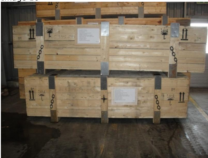
Image shows: Boxes over 2000 kg with an angle bracket.
