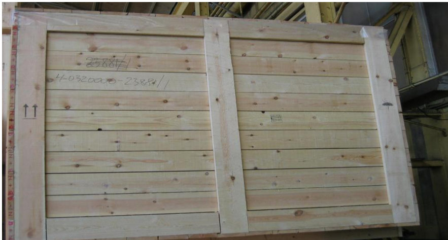
End of the box with additional stiffening elements
