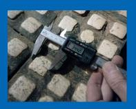
After 16 weeks of operation, wear measurement revealed only 10-13% wear on the ceramic inserts and no visible cracks or chipping
