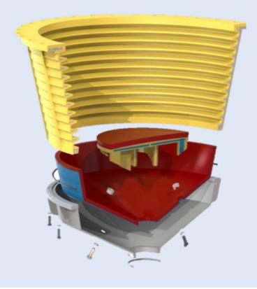
At the heart of this gravity separation technology is the Knelson™ concentrating cone. And our new patented GX model delivers impressive recovery enhancements. By incorporating an advanced distribution of fluidisation water across the entire concentrating cone, the Knelson™ GX significantly improves recovery.
