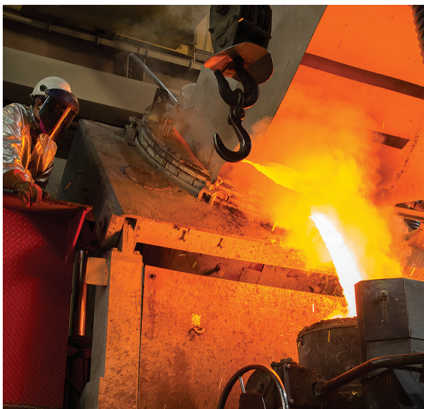
Standard bronze pour from furnace to ladle in our FLSmidth foundry for EXCEL parts
