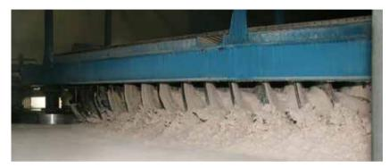
Deliquoring, cake washing and cake drying are performed during one pan revolution. Counter-current cake washing in up to three washing steps with exact separation of the filtrates is done with excellent results at minimum water consumption. For additional reduction of cake moisture, the filter can be equipped with a steam hood located in the drying area.
