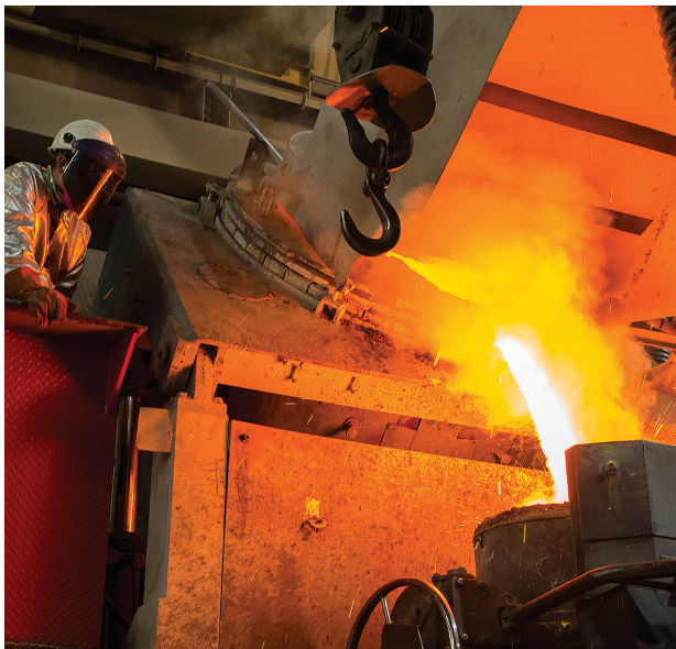
Standard bronze pour from furnace to ladle in our foundry for EXCEL parts, located in Pekin, Illinois, USA
