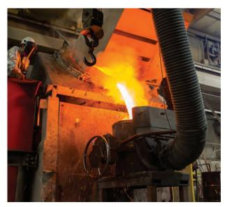
Standard bronze pour from furnace to ladel in our foundry for EXCEL parts, located in Pekin, Illinois, USA
