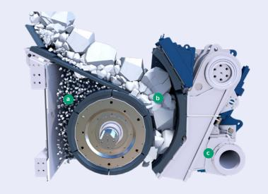
Fine particles fed into the crusher are screened by the integrated static grizzly and bypassed through the crusher housing (a). The coarse feed material fraction is continuously crushed between the oscillating roll and the jaw until the product exits the crushing chamber at the bottom (b). The integrated hydraulic gap setting system allows for wear liner compensation, release of uncrushable material like tramp metal and gap adjustment (c).
