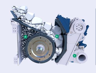
Fine particles fed into the crusher are screened by the integrated static grizzly and bypassed through the crusher housing (a). The coarse feed material fraction is continuously crushed between the oscillating roll and the jaw until the product exits the crushing chamber at the bottom (b). The integrated hydraulic gap setting system allows for wear liner compensation, release of uncrushable material like tramp metal and gap adjustment (c).
