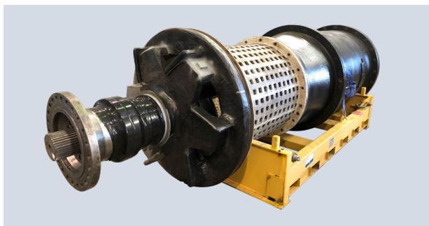
Screenbowl Rotating assembly on transport frame, ready for protective wrap
