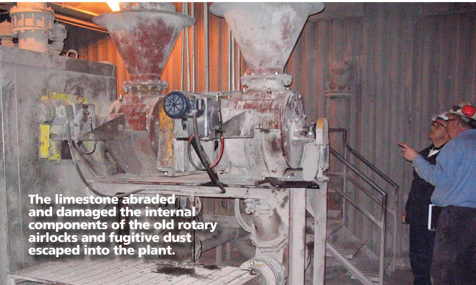
**The limestone abraded and damaged the internal components of the old rotary airlocks and fugitive dust escaped into the plant.**
