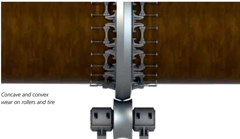
Concave and convex wear on rollers and tire
