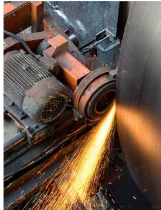
Thrust face grinding
