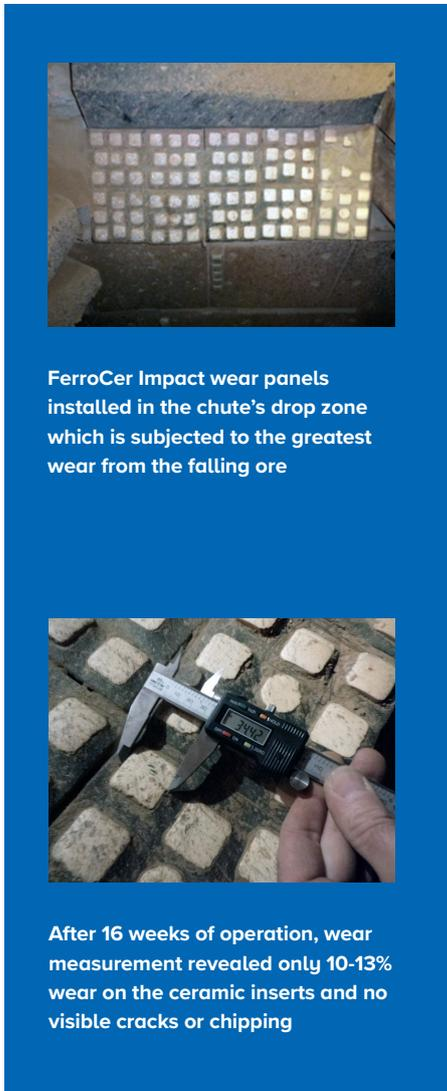
**FerroCer Impact wear panels installed in the chute’s drop zone which is subjected to the greatest wear from the falling ore**
