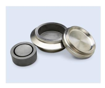
Tungsten carbide grinding heads are made by sintering carbide powder with a cobalt metal powder binder. Tungsten carbide is the grinding head of choice for many laboratories where elemental contamination is limited to just two principal contaminants: tungsten and cobalt.
