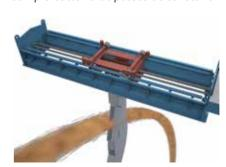
speed through a falling stream of slurry or free flowing solids. Correct cutter geometry design ensures radial cutter edges accurately cut a fixed portion of the stream.
