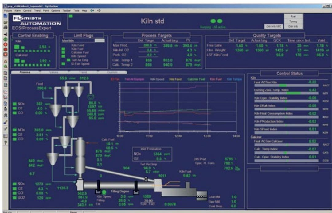
Automated control ensures a timely and correct response to process changes. The result is a stable pyro system and reduced NO<sub>x</sub> emission.
