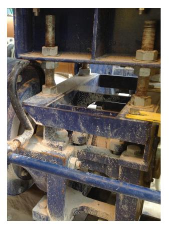
Nuts have to be adjusted individual to lower conventional motor mounts.
