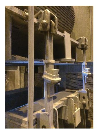
Removing the wedges allows the motor mount to move up and down with the ram.
