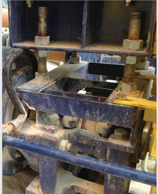
Nuts have to be adjusted individual to lower conventional motor mounts.
