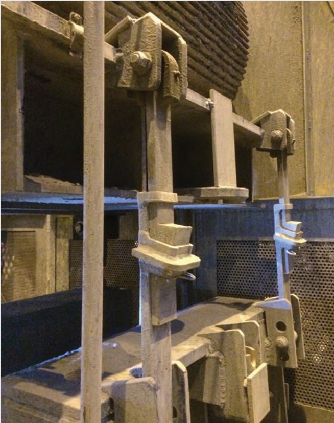
Removing the wedges allows the motor mount to move up and down with the ram.
