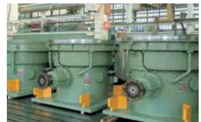
Bevel-planetary gear type.
