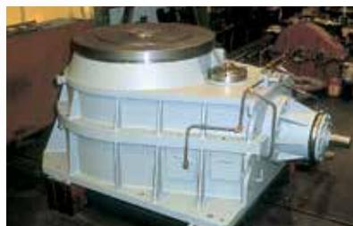
Bevel-helical gear type.
