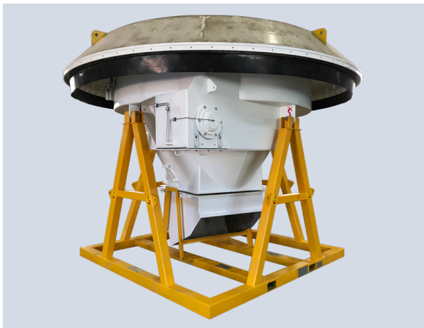
SPD15 mounted on the installation frame
