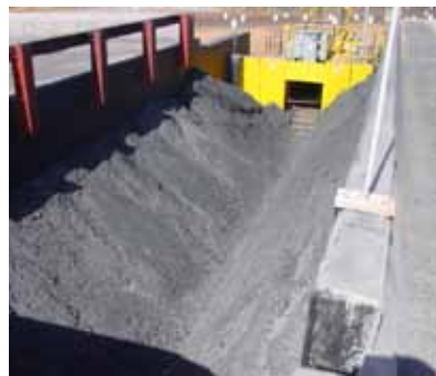
Reclaim Feeder for use with side tip trucks
