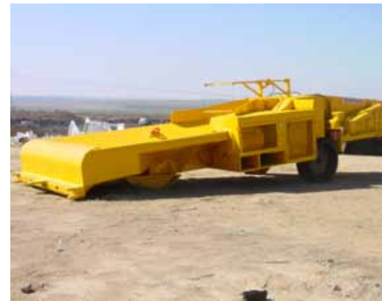
Coarse Coal Breaker assembly
