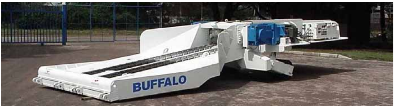
Low Seam Feeder Breaker
