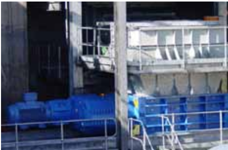
Primary Tip Sizer in Maintenance Position
