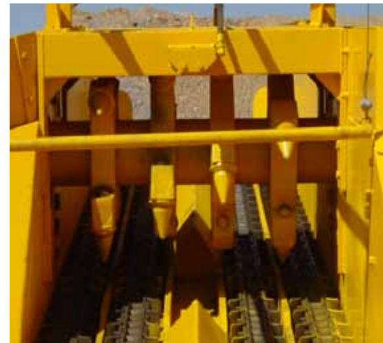
Coarse Coal Breaker assembly
