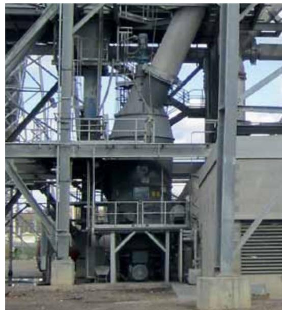
FLSmidth Atox mill with MAAG™ coal mill gear unit
