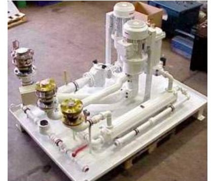
The lubricating system is delivered as one unit on a foundation plate and designed for mounting either on the left or the right side of the gear foundation.
