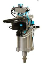
Our standard offering includes FESTO $^{\text{\tiny{M}}}$  actuators, which receive data from the level sensor and adjust the dart valve position to maintain slurry levels. All actions taken by the control system are based on these measurements, so accuracy is imperative for optimal performance.
