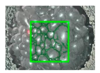
With flotation imaging sensors, operators now can monitor and measure flotation performance metrics such as overflow velocity and froth height on an individual cell basis. This ensures the operator can take corrective action for the appropriate cell. It also allows the automated process control (APC) system (if installed) to control the plant in a more stable manner, and reduces variances around the overall mass pull target.
