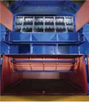
Opening for dismantling breaker plates and outlet grate adjustment
