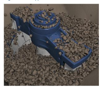
Wear plates for high-abrasion applications comprise a spider hub and optional underside liner, which completely cover the spider to protect assembly from wear, even in the most abrasive applications.
