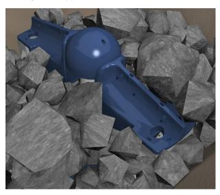
Blocky feed often leads to bridging. The ridgeline design of this wear plate style features a prominent peak that will split feed around the plates, improving flow into the crushing chamber.
