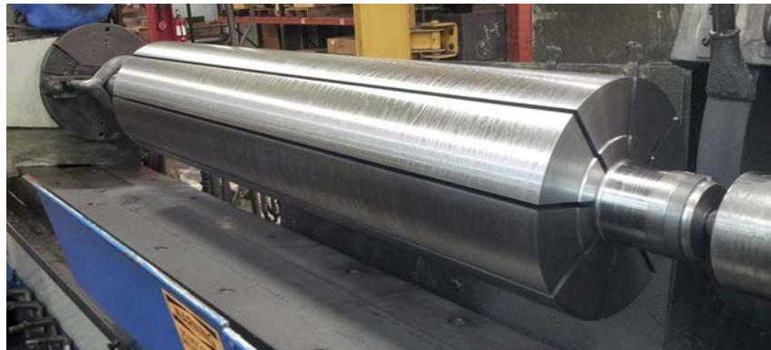
Compressor rotor mounted for reslotting
