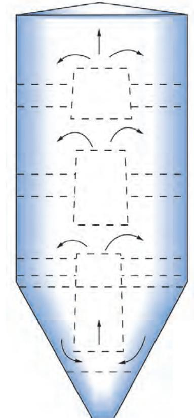
*The column blender can accommodate different volumetric batch sizes.*
