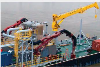
Starting with a range of four basic sizes, FLSmidth can supply the right DOCKSIDER ship unloader for any terminal – whether you're unloading river barges or Handymax bulk vessels, and whether you're conveying to an adjacent belt conveyor or through a 1200 m (4000 ft) pipeline.
