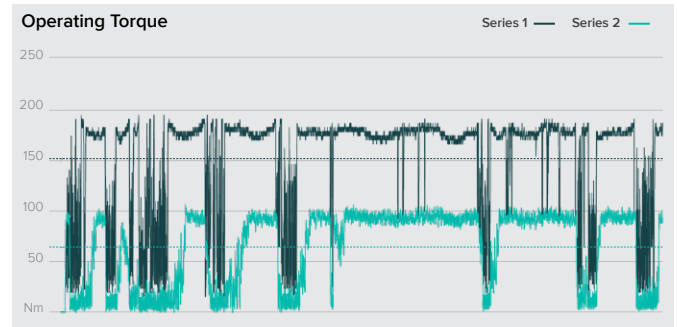
Above: Series 2 demonstrates a more-consistent operating torque
