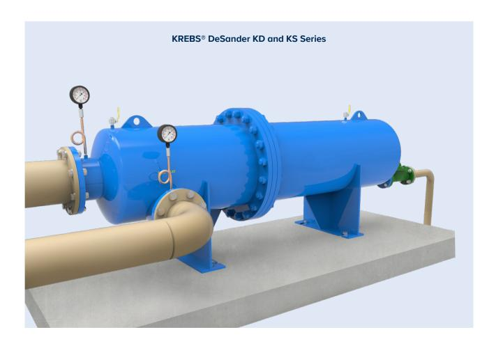
We produce different types of cyclones and desanders to meet your specific requirements. Each type comes with a choice of sizes (from 2 - 30 in. diameter), internal fittings and linings. You can choose to leave your unit unlined, line it with vulcanized gum rubber, or line it with replaceable gum rubber liners, according to your budget and preferred life of the unit. For ease of installation, all our units can be mounted horizontally, vertically or at any angle in between.
