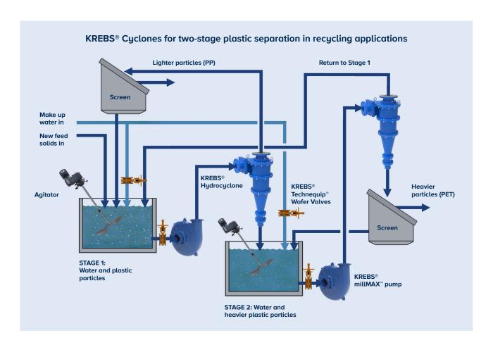
Plastics separation and heavy trash separation are carried out in two steps with two different models of cyclone. If you need very clean heavy and light plastic, a two stage counter current system can be added.
