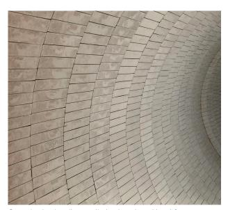
Ceramic alumina tiles applied to beach and bowl for wear resistance
