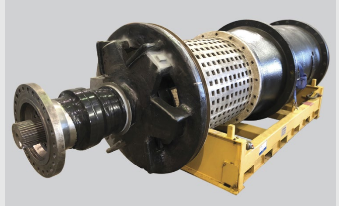
Screenbowl Rotating assembly on transport frame, ready for protective wrap
