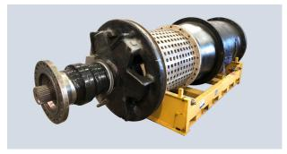
Screenbowl Rotating assembly on transport frame, ready for protective wrap
