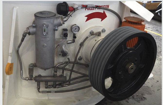
FC1200 Lubrication System (LS) assembly and driven pulley
