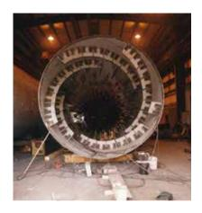
transfer. The internals (starting from the feed end) consist of: feed advancing spirals to minimize backspilling, straight lifters bolted to angle brackets which are welded to the shell, and a section of bare shell at the discharge end to minimize dust entrainment
