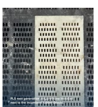
The ligament size measured at the end of panel life showed that the polyurethane panels installed at the feed end and middle section of the screen had wear rates that were comparable with the rubber panels. At the discharge end, it had a significantly lower wear rate than the rubber media.
