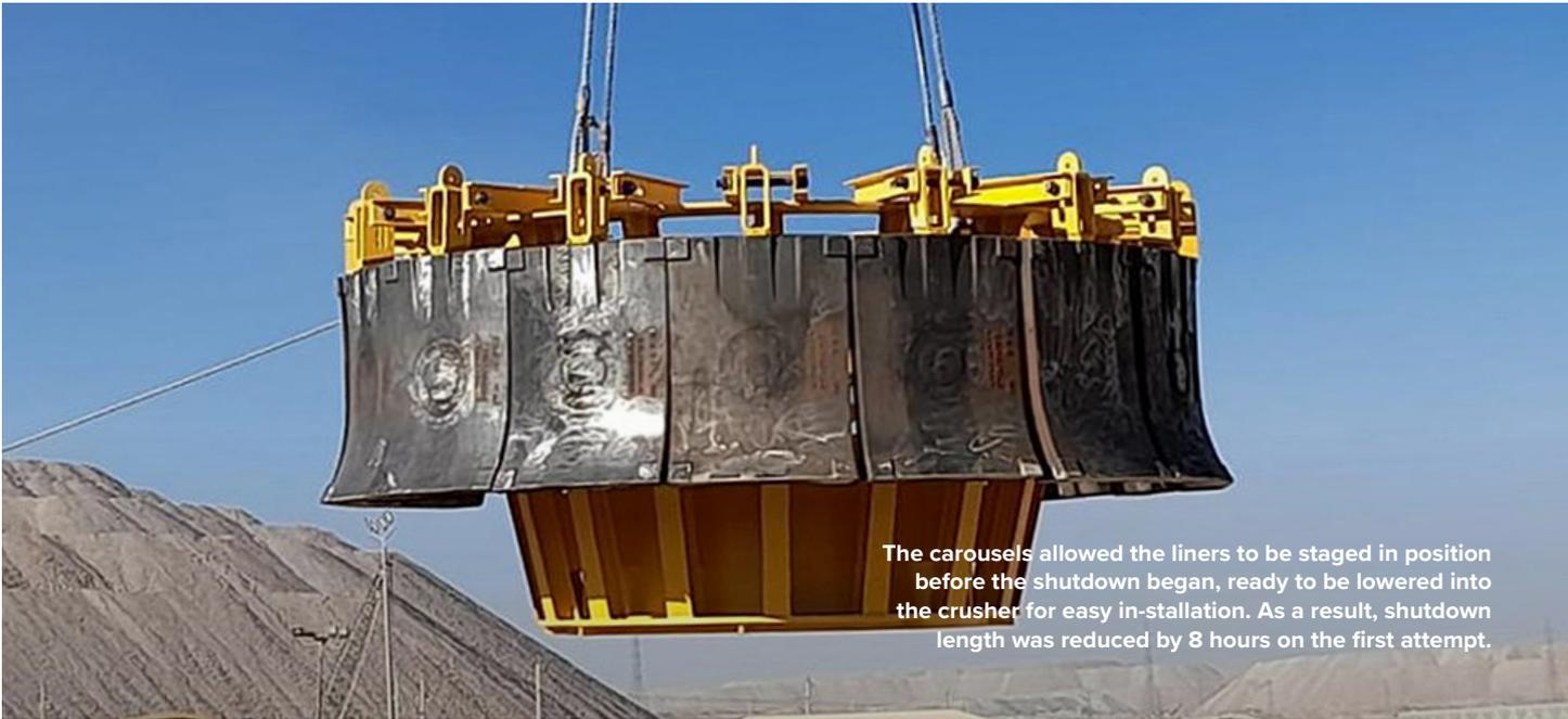
The carousels allowed the liners to be staged in position before the shutdown began, ready to be lowered into the crusher for easy in-stallation. As a result, shutdown length was reduced by 8 hours on the first attempt.
