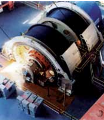
Ø 6.0 m Double Drum Hoist, 19 tonne payload - Moab Khotsoeng
