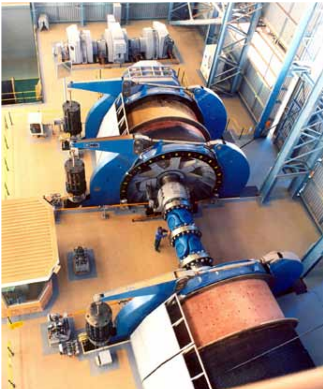
Ø 5.1 m BMR Hoist with Hookes Joint Coupling - South Deep
