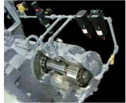
Type M pump pressurized seal and shaft bearing assembly
