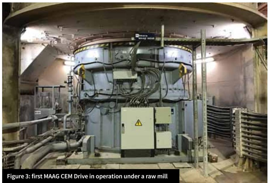
**Figure 3: first MAAG CEM Drive in operation under a raw mill**
