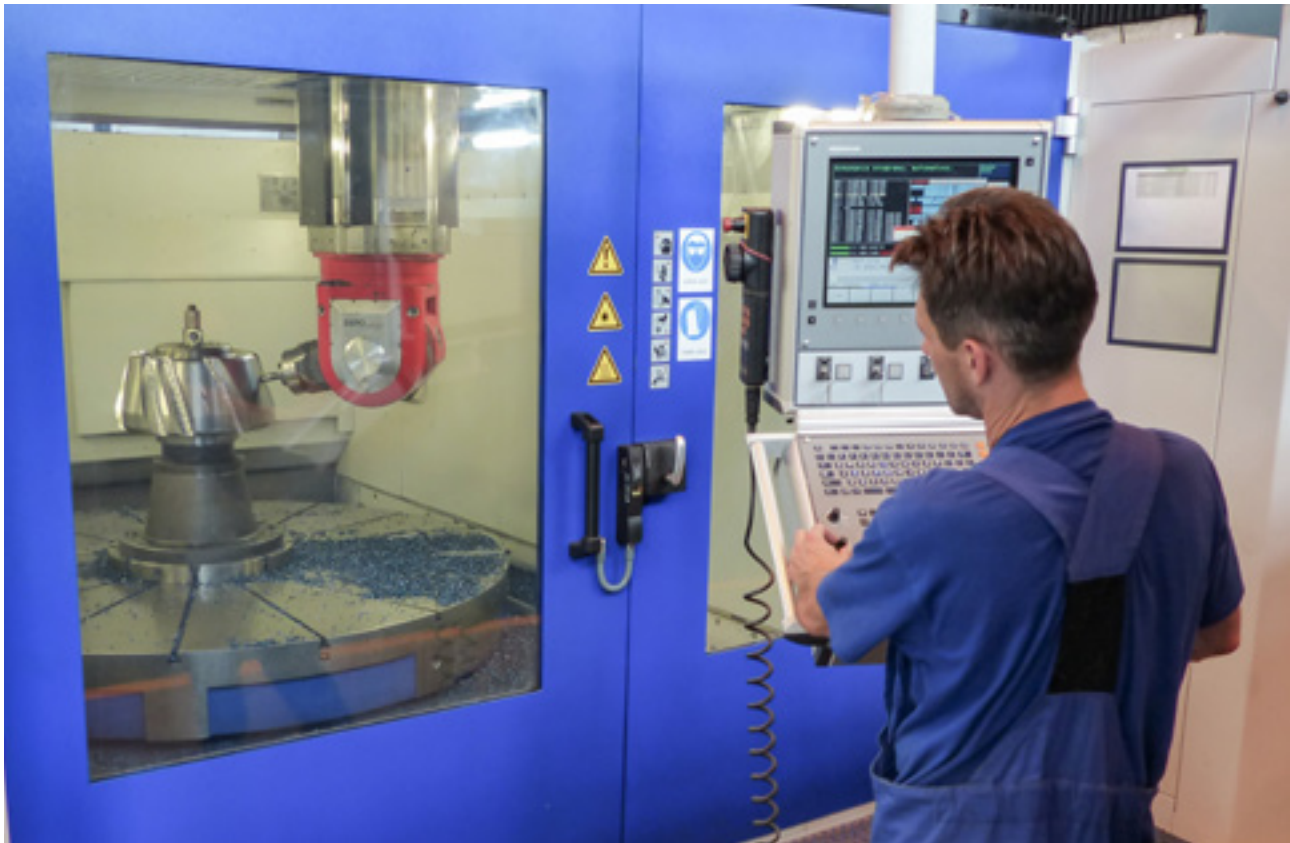
PRODUCTION OF A BEVEL PINION BY FIVE-AXLE MILLING MACHINE
