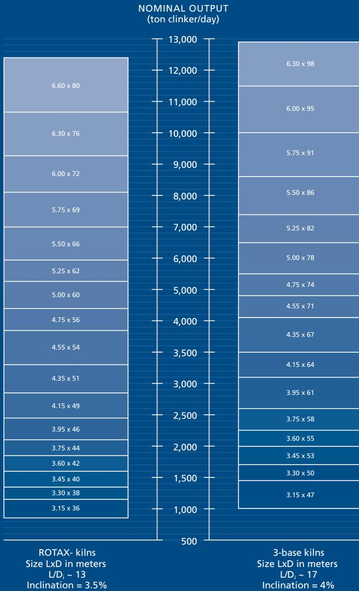
Kiln length is variable within a range and can be designed for special cases. The nominal output is based on normal clinker quality and kiln volumetric loading of 5.0 ton/day/m<sup>3</sup> for 3-base kilns and 5.3 ton/day/m<sup>3</sup> for ROTAX-2 kiln. The potential output of a kiln also depends on the burnability of the raw materials. The kiln rotational speed is designed for 5.0 rpm (revolutions per minute) with a nominal speed of 3.6.
