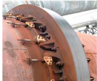
*Kiln tyre with tangential suspension*
