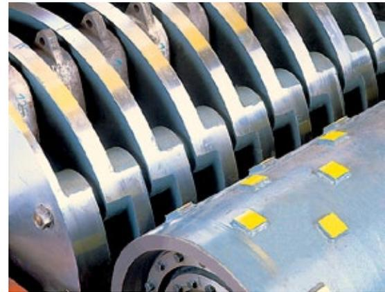
*Sandwich construction hammer rotor and part of inlet roller.*
