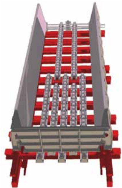
Impact and supporting rollers are fitted below the aprons.
