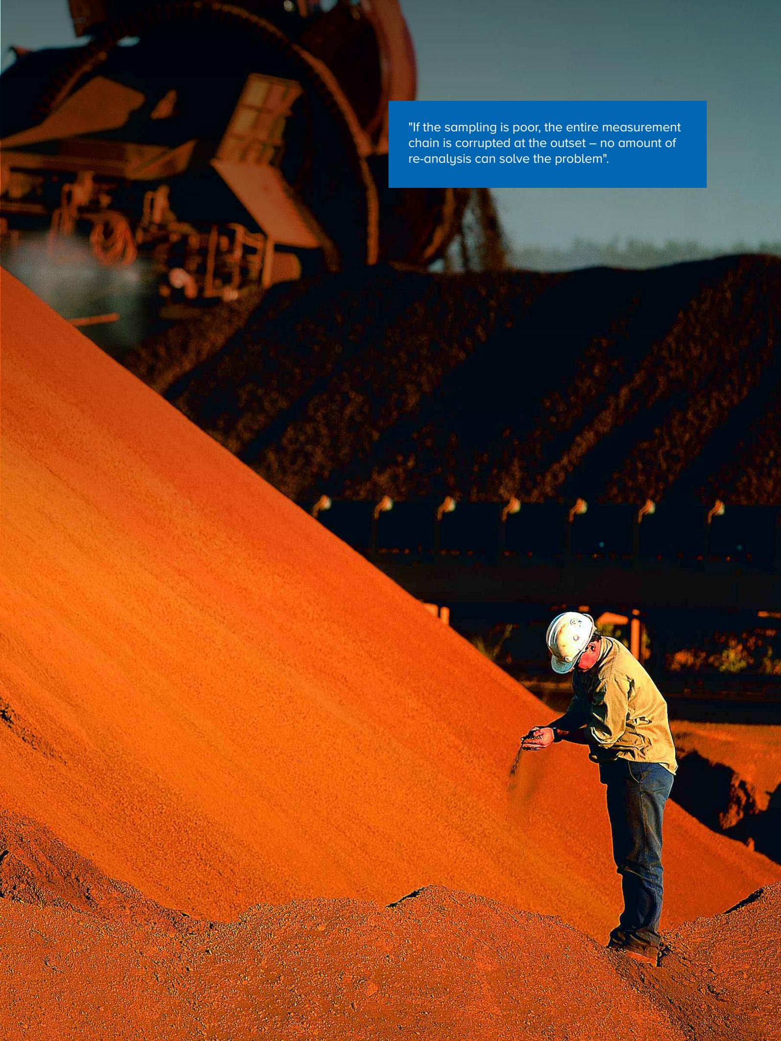
A photograph of a worker in a white hard hat and a yellow safety vest standing on a large pile of bright orange material, likely iron ore. The worker is holding a small tool and appears to be sampling the material. In the background, there are large industrial structures and more piles of the same material under a clear sky. A blue text box is overlaid on the upper right portion of the image.
