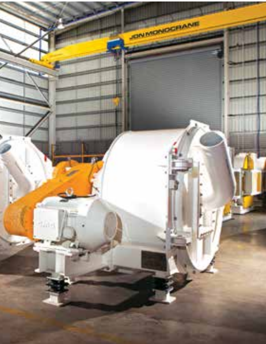
HFC™1300 Horizontal Fine Coal Centrifuge (Front)
