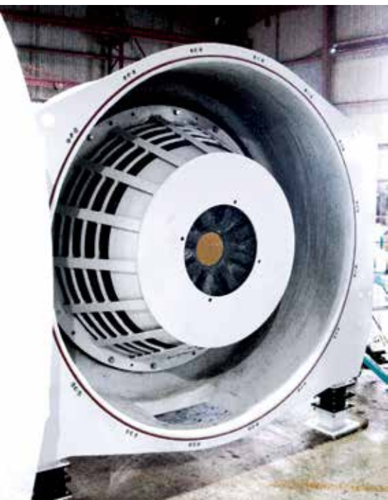
HFC™1300 Horizontal Fine Coal Centrifuge Basket (internal)
