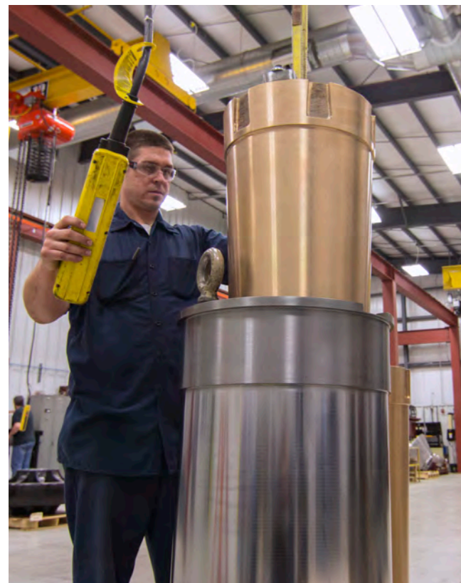
Installing the Symons® inner eccentric bushing
