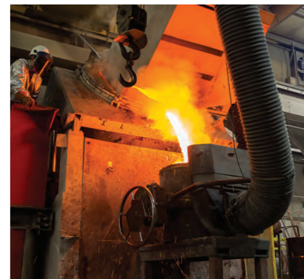
Standard bronze pour from furnace to ladle in our foundry for EXCEL™ parts, located in Pekin, Illinois, USA
