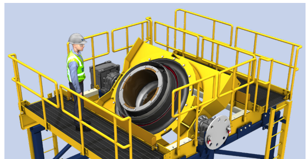
Gearbox driven rotating mechanism for full 360° rotation
