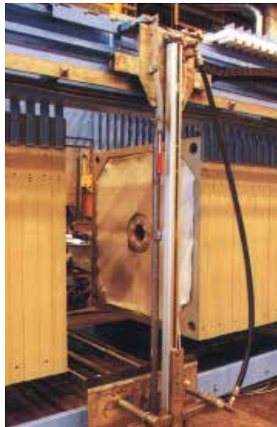
Automatic plate washer on overhead beam filter
