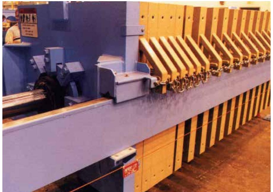
Above: ALP™ Shifter with standard Heavy Duty SS Investment cast shifting carriage for reliable shifting of the heaviest plates.
