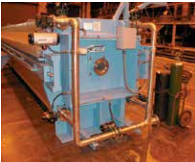
Process control manifolds for manual or automated slurry feed, filtrate discharge, cake washing (when required) and air blow down
