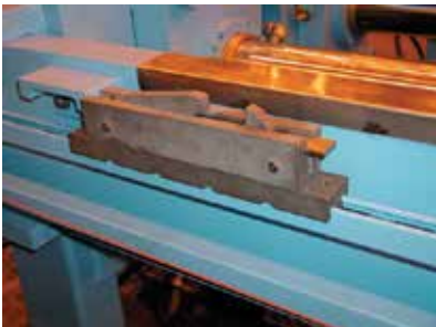
Above: ALP™ Shifter with standard Heavy Duty SS Investment cast shifting carriage for reliable shifting of the heaviest plates.
